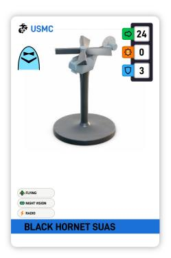
This fist-sized drone is used for reconnaissance by Marines. Cheap, light, and effectively disposable, the Black Hornet is equipped with night vision, thermal, and optical cameras as well as a laser range-finder, allowing Marines to use the drone for target acquisition and observation.
